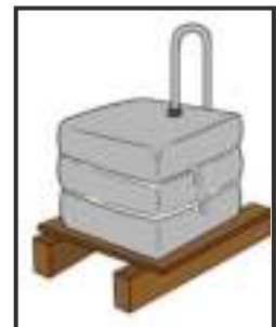
Insulate the cold water tank
